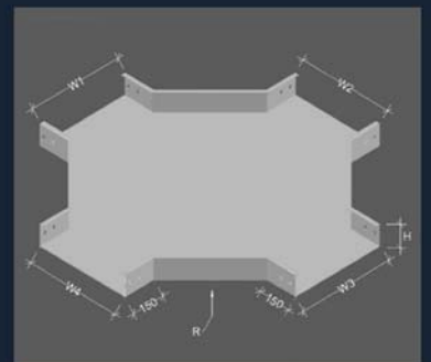
Horizontal Cross Diagonal Duct - Type
